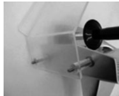
2. Attach the hand guard.
